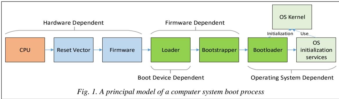
Fig. 1. A principal model of a computer system boot process
