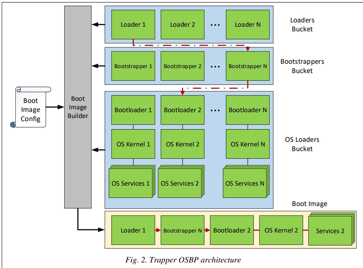
Fig. 2. Trapper OSBP architecture
